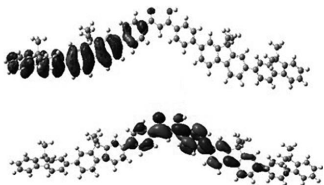
Figure 9. Calculated HOMO (top) and LUMO (bottom) distributions for the model compound of PFO-dbm.
